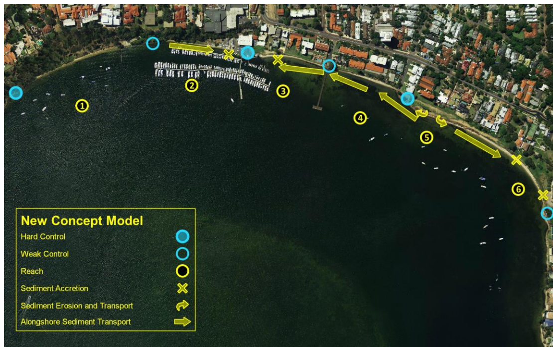
Figure 11: Conceptual Model of Claremont Foreshore Dynamics
