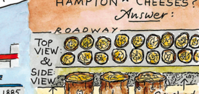
JARRAH 'LONG ROUNDS' This formed a hard road surface used for the Perth-Fremantle road
